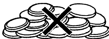
Example of stacked and jumbled batteries
